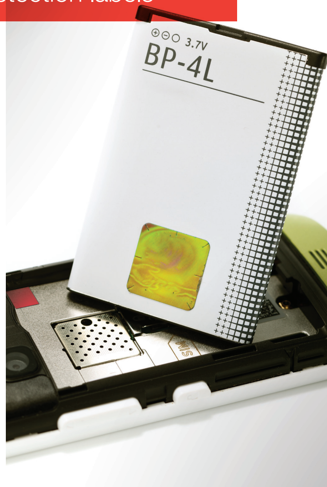
Water detection label in battery housing changes color irreversibly upon contact with water.
